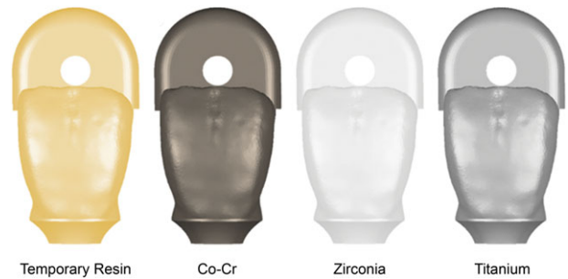
Figure 1 CAD design simulating different crown materials with the pull handle for the pullout test.
