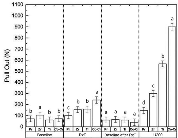
**Figure 4** Pullout retention values as a function of mean and 95% confidence interval. For U200 and RelyX Temp NE, Co-Cr evidenced higher pullout strength compared to other materials. Groups without cement demonstrated similarity regarding to pullout strength data for all crown materials, except Zr baseline. Different letters indicate significant difference between groups ( $p < 0.001$ ).
