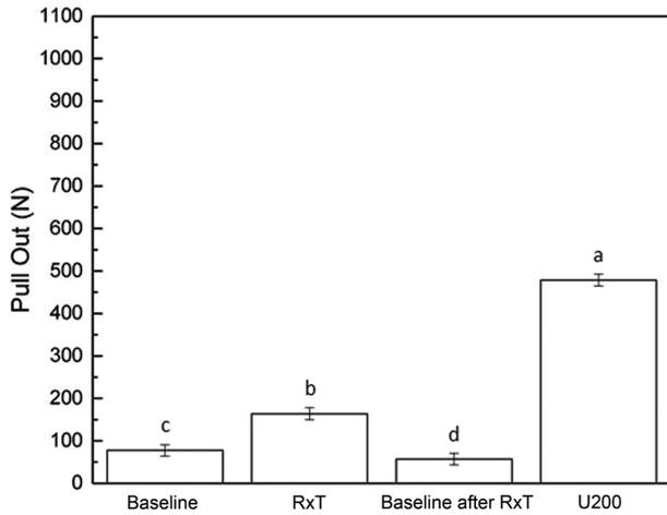
**Figure 2** Pullout retention values as a function of mean and 95% confidence interval. U200 group evidenced higher pullout strength compared to other groups. Different letters indicate significant difference between groups ( $p < 0.001$ ).
