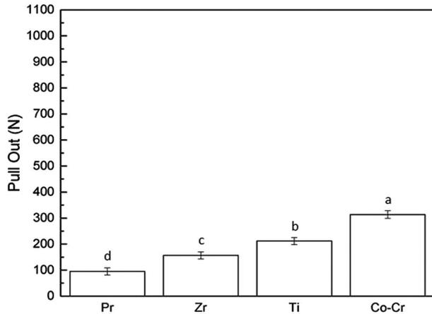
**Figure 3** Pullout retention values as a function of mean and 95% confidence interval. All crowns materials were significantly different. Different letters indicate significant difference between groups ( $p < 0.001$ ).
