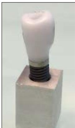
**Fig 4** Test specimen after implant placement into aluminum blocks and abutment adaptation.
