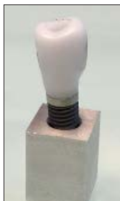
Fig 4 Test specimen after implant placement into aluminum blocks and abutment adaptation.
