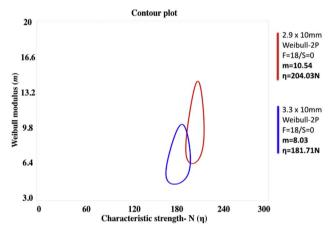
Fig. 2. Contour plot showing "m" as an indicator of reliability (Weibull modulus) vs. characteristic strength  $(\eta)$ , which indicates the load in which 63.2% of the specimens of each group may fail. The overlap between groups indicates they are homogeneous.
